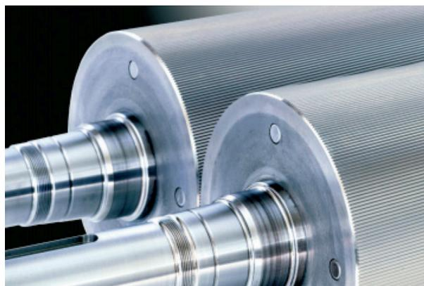
Figure 2. Detail of grooved cylinders. Source: [https://www.buhlergroup.com/europe/es/downloads/Roll-Service-for-Roller-Mills\\_en.pdf](https://www.buhlergroup.com/europe/es/downloads/Roll-Service-for-Roller-Mills_en.pdf)
